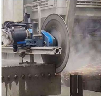
HF Wall Saw Cut Steel Rebar
