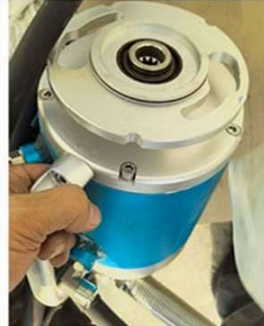
Full Water Seal HF Motor
