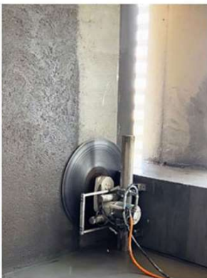
Wire Saw Head Unit with High Frequency Motor
