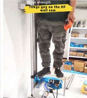
Saw Head Strength Test
