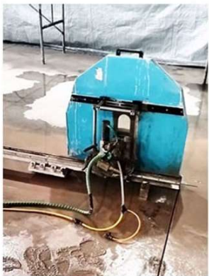
Wire Saw Head Unit with High Frequency Motor
